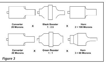
Depending on the material and ultrasonic process utilized, different amplitudes will be necessary. Amplitude can be measured in either thousandths of an inch or microns (0.001'' = 25 microns).
